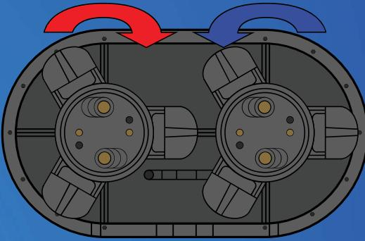
Opposite rotating heads mean the operator does NOT fight the machine.
